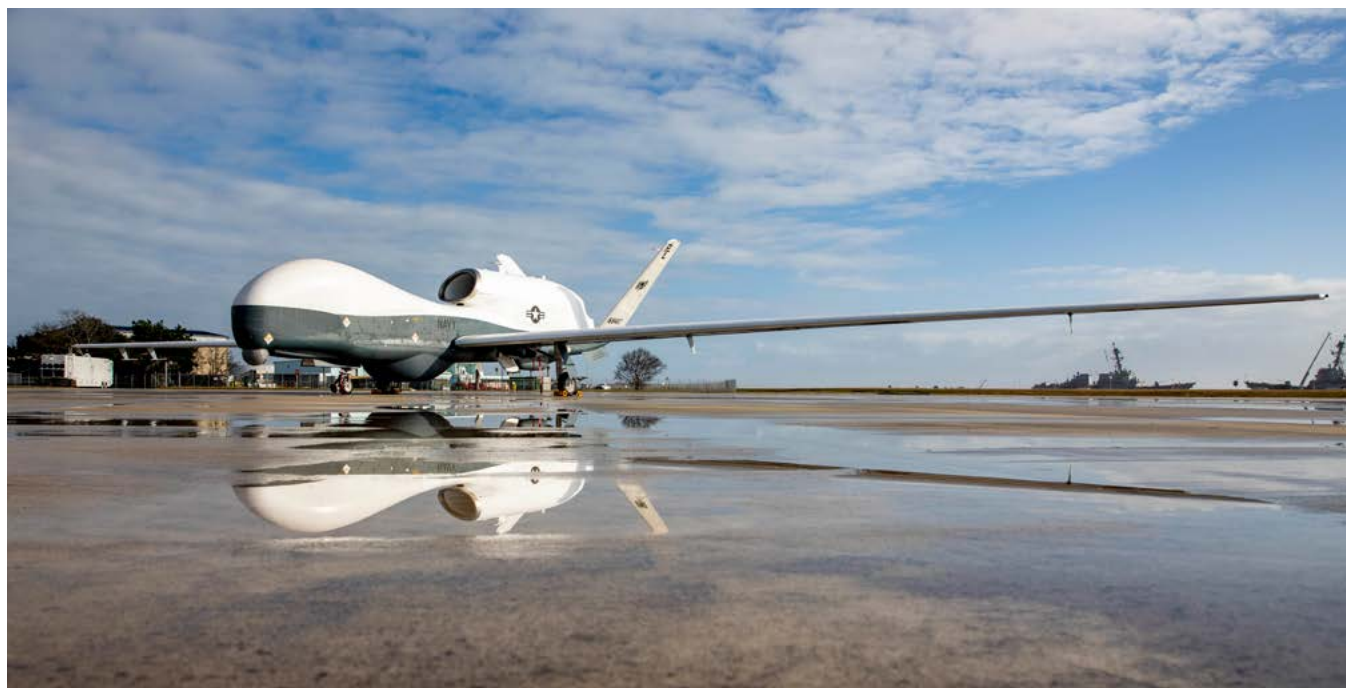
An MQ-4C Triton Unmanned Aircraft System (UAS) assigned to Unmanned Patrol Squadron 19 (VUP-19), at on the flight line at Naval Station Mayport, Florida, December 16, 2021. (US Navy photo by Mass Communication Specialist 2nd Class Nathan T. Beard)
