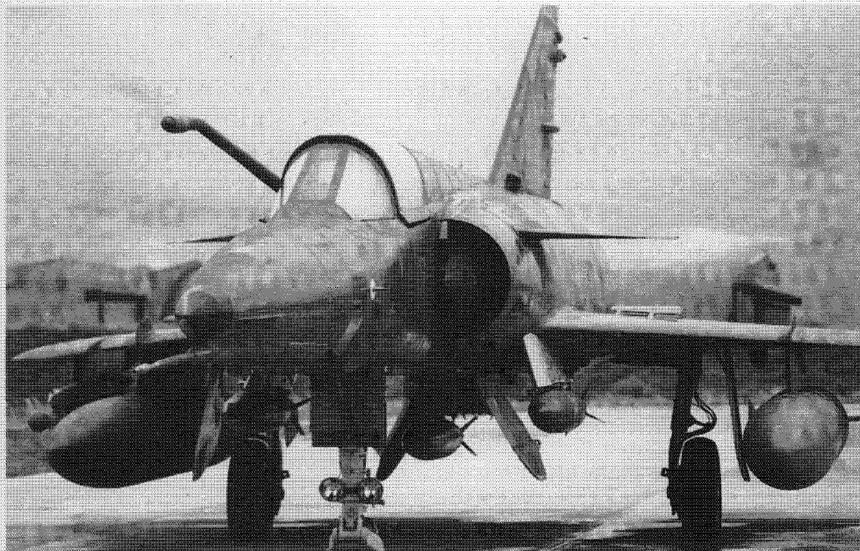
Figure 2. The Cheetah. This modified Mirage-III is built at Armcor's Atlas Aircraft subsidiary.
