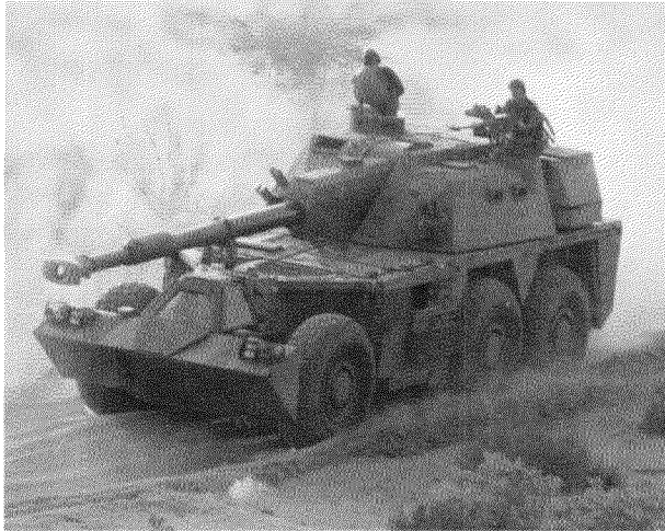
Figure 4. The G-6 self-propelled howitzer, built by Armscor's Lyttleton Engineering subsidiary.
