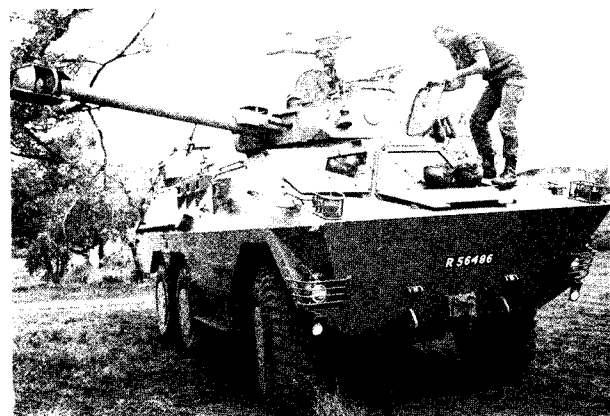
Figure 9. Two Versions of the South African-Designed and Manufactured Ratel Infantry Fighting Vehicle. Top: The Ratel 60 with a 60-mm mortar. Bottom: The Ratel 90 with a 90-mm gun. [redacted] International Defense Review ©
