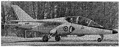
Power: 2 turbofan engines creating about 3,000 lbs thrust each length: 40 ft Wing span: 30 ft Takeoff weight: about 10,000 lbs Speed: Mach 0.9 Takeoff run; less than 1,600 ft
