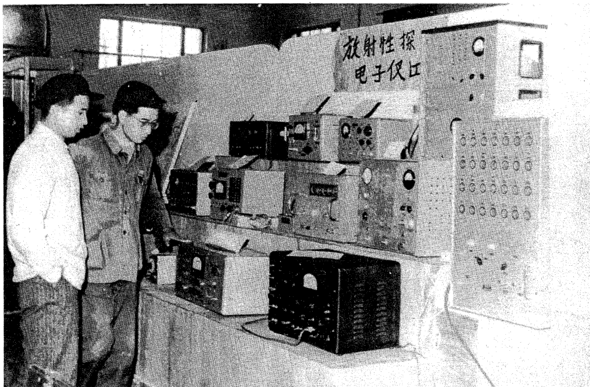
Figure 15. Counting equipment for the detection of radioactive tracers.
