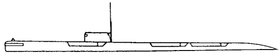
Drawing of "E-I" Class SSGN with missile launching tubes in stowed position.
