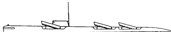
Drawing of "E-I" Class SSGN with missile launching tubes in elevated position.
