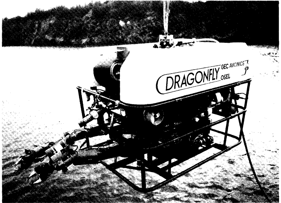
British-built remotely operated vehicle used for subsea repair and maintenance.
