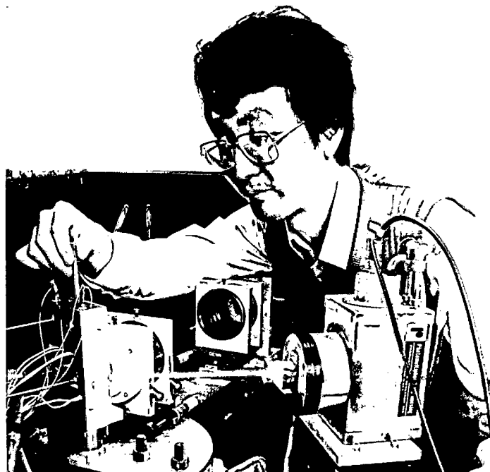
Takahiro Sato, a guest scientist from Osaka University, Japan, uses the temperature-jump light scattering technique to record the phase separation behavior in molecules.
