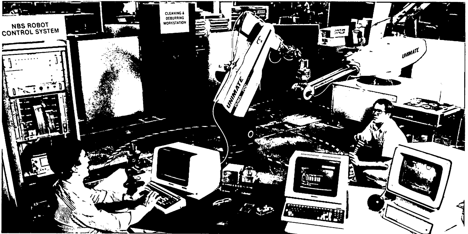
Research engineers Karl Murphy (foreground) and Rick Norcross study the performance of an experimental parts-deburring station at the NBS Automated Manufacturing Research Facility.
