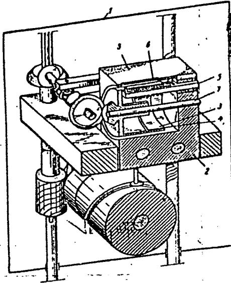
1--vacuum chamber; 2--mechanical scanner; 3--rotating drum; 4--helical slot; 5--collector; 6--rectangular slot; 7--drum axle
