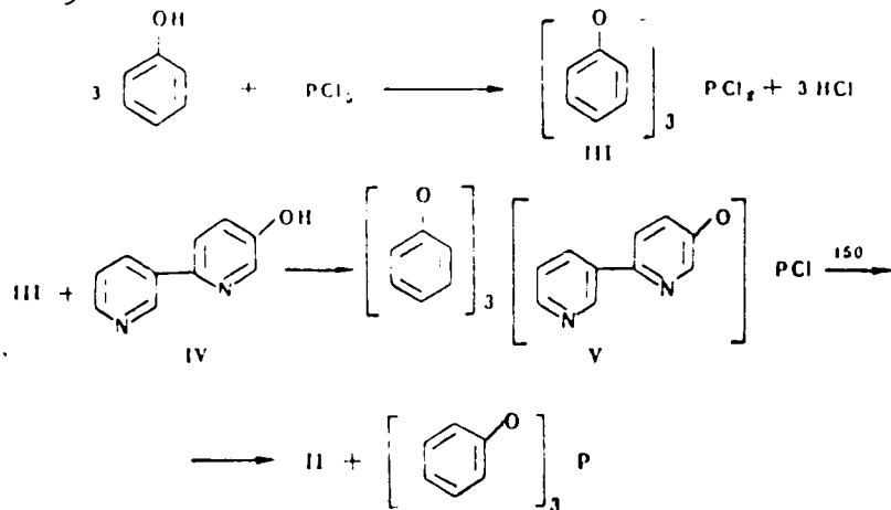
and heating of V to  $150^\circ$  produced bipyridyl II, as indicated by UV and IR spectra. The chlorination of piperidine was carried out under similar conditions, and 3-chloropyridine was obtained. Orig. art. has: 2 figures.
