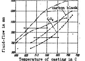
The use of carbon black or hexachloroethane coatings considerably improves the degree of mold filling, permits lowering of the casting temperature, increases the density of castings, and prevents the formation of hot cracks in the castings. Coating of molds with hexachlorobenzene had little or no effect either on the properties of the alloy melt or the quality of the castings. P. F. Odiny participated in the experimental work. Orig. art. has: 12 tables and 2 figures.
