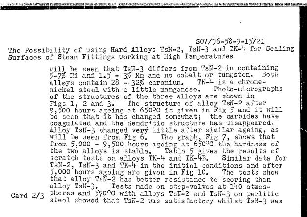
sov/96-58-9-15/21 The Possibility of using Hard Alloys TsN-2, TsN-3 and TK-4 for Sealing Surfaces of Steam Fittings working at High Temperatures The reason may be that, of the two alloys, TsN-3 has a coefficient of expansion nearer to that of the base metal.
