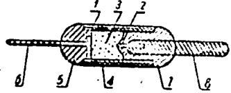
Figure 2. 1---anode (Pt); 2---cathode (Pt);
