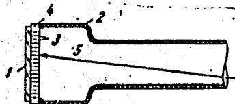
1 - Receiving piezoelectric plate; 2 - Converter body; 3 - Thin metal lead-in; 4 - glass plate; 5 - electron beam.
