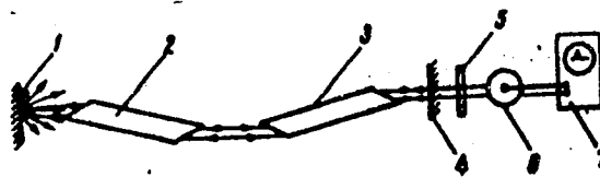
Fig. 1. Diagram of experiment. 1 - Scatterer, 2,3 - ruby crystal, 4 - mirror, 5 - filter, 6 - photocell, 7 - oscilloscope.
