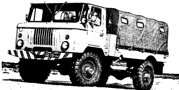
Figure 10. GAZ-66 2-ton, all-wheel drive military truck. [redacted]
