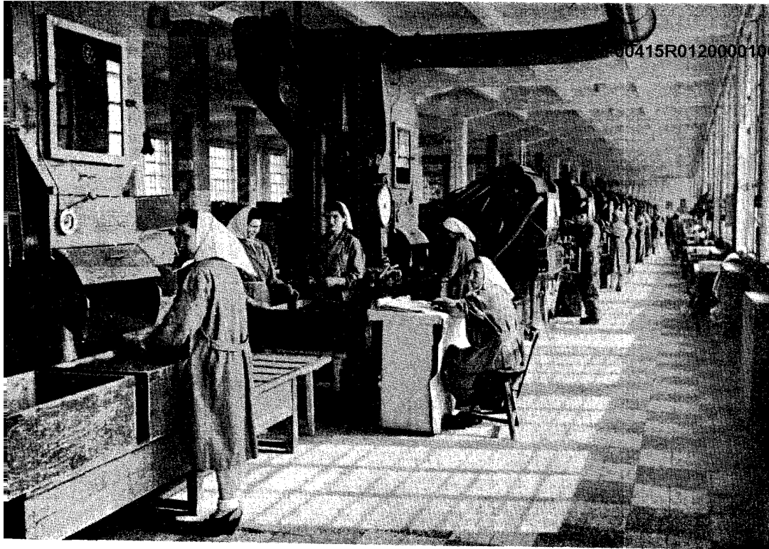
The cigarettes are conveyed to the packing in special frames
