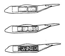
The CN-235 will be capable of transporting two 2.23-meter palettes, or four LD-3 containers, or five LD-2 containers.
