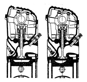
One of the problems in developing the TOP engines was to utilize the advantages of thermodynamic optimization under part-throttle conditions without losing maximum engine performance compared with the production engines. By carefully designing the composition of the air-fuel mixture along the full-throttle line and carefully setting the ignition timing in the entire throttle and rev range the requirement could be met.
