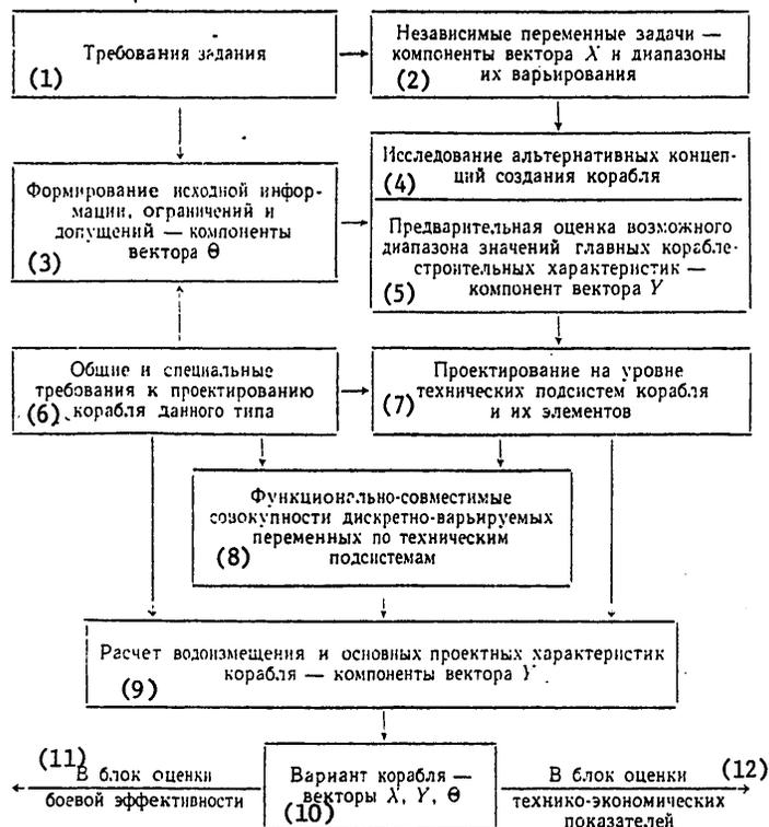
Figure 2.1. Schematic diagram of the solution of the problems of the engineering design block during the AD process
