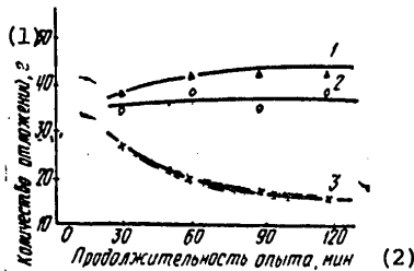
Figure 2. Effectiveness of Reagents Depending on Time of Contact With Deposits of Solid Hydrocarbons and Asphaltic-Resinous Substances: 1--deposit soluble fraction (reagent's dissolving action); 2--deposit dispersed fraction (reagent dispersing action); 3--deposit insoluble fraction on metallic net
