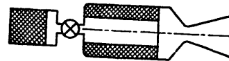
Figure 11.4. Schematic of the solid-fuel rocket engine with thrust regulation by variation of the feed of the initial gaseous component
