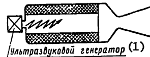
Figure 11.2. Schematic of a solid-fuel rocket engine with thrust adjustment by varying the vibrational characteristics of the chamber
