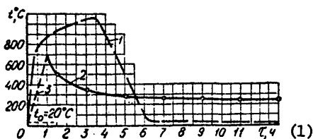
Figure 66. Graphs of the temperature variation 1 -- in the center of the fire; 2 -- fragments of the structural elements after collapse; 3 -- surfaces of the structural elements before reaching the limit of their fireproofness
