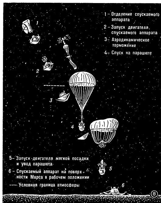
Figure 8. Landing pattern of the reentry vehicle of the "Mars-3" station.
