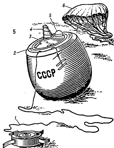
Figure 5. Releasable Apparatus of the Station "Venera-8" on the Surface of Venus
