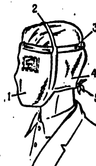
Fig. 121. The PTM-1 fabric dust mask on: 1--body; 2--cross strap; 3--rubber band; 4--strengthening; 5--straps.
