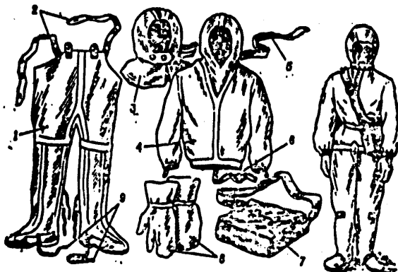
Fig. 124. The L-1 light protective suit: 1--trousers with boots; 2--shoulder straps; 3--helmet liner; 4--shirt with hood; 5--neck flap; 6--crotch band; 7--bag; 8--two-finger glove; 9--straps.
