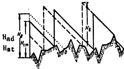
Fig. 5.12. Determination of limits of zone of possible positioning of petroleum pumping stations with rounding off of their number in the greater direction.
