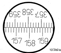
Fig. 10. Reading of limbus = 157.95°
