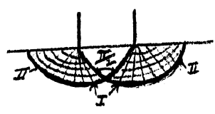
Fig 7 - Diagram of Sliding Surfaces in Frozen Soils For a 130r Load (p 53)
