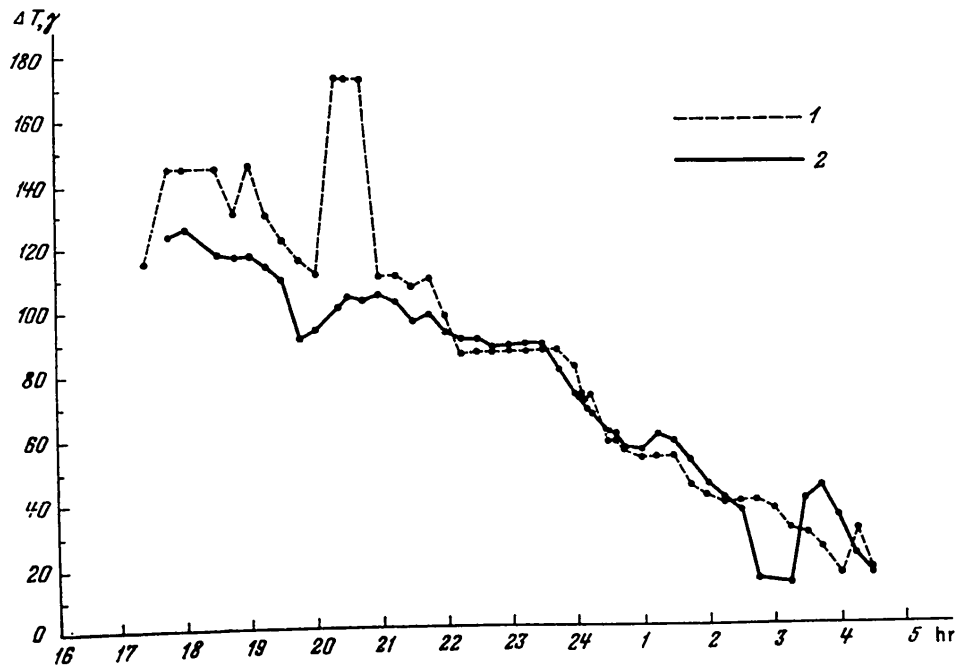
Fig. 2. Change of Intensity of Full Vector \Delta T on March 11-12, 1958 (1- Readings of SG-45 29153; 2- readings of observatory magnetograph)
