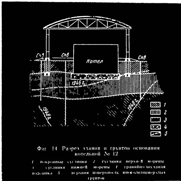
Boiler House No. 12, Sanitation Plant Section Through the Structure and the Foundation Bearing Layer. Ckb denotes bore hole
