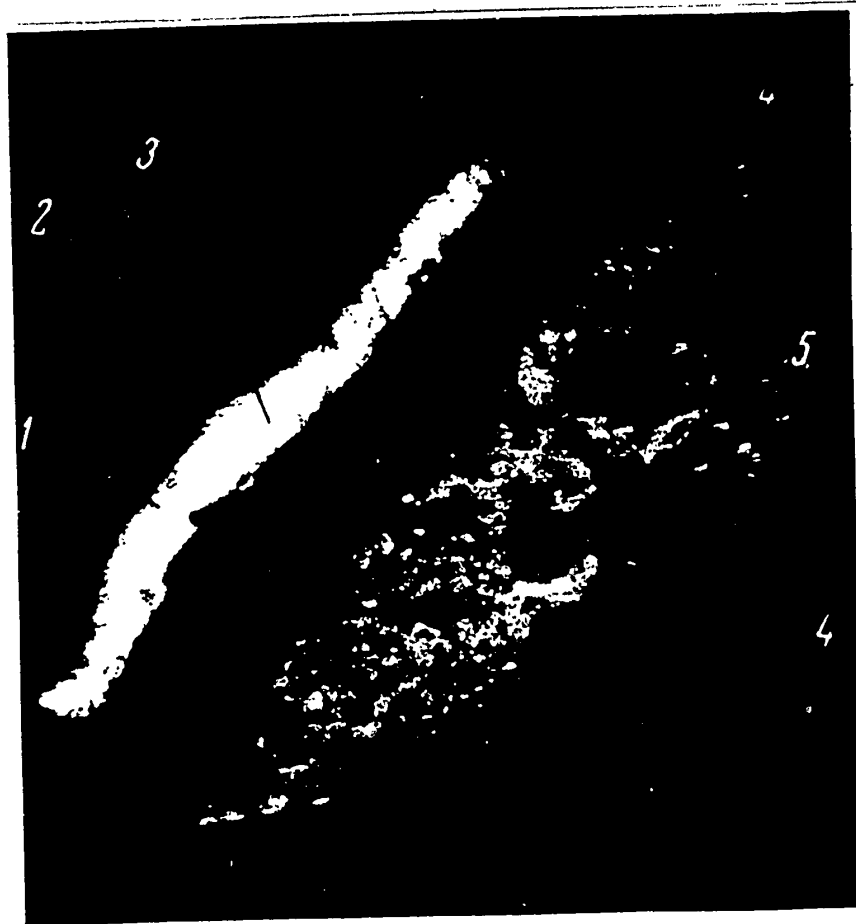
Fig. 53 - Friction Surface of Brake Shoe made of Plastic No. 22 after Operation in a Chamber Brake. Cross Section of Polished specimen, not etched, \times 200 (V. M. Gudchenko).
