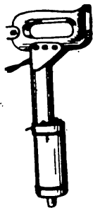
Fig. 302 - Electric Heating Device for Riveting Explosive Rivets
