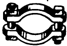
Fig.251 - Clip for Fastening a Hose to the Shank of a Quick- Release Coupling
