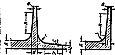
Fig.47 - Design of Junctions in Aluminum Alloy Castings
