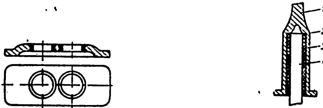
Fig.18 - Pouring Anti-Friction Bronze Into a Silumin Detail. Fig.19 - Casting a Bushing Into a Cylinder: 1) Gate; 2) Casting; 3) Bushing; 4) Core Cutter.
