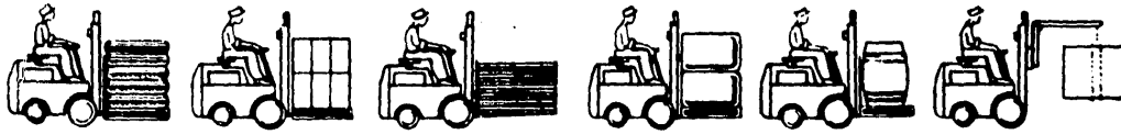
Teamed with pallets or dunnage, equipped with regular forks or home-made variations, fork lift trucks successfully handle most materials.
