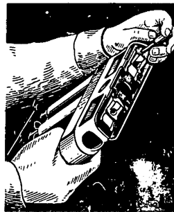
FIG. 39. LOADING SIGNAL FLARE LAUNCHER WITH IGNITERS
