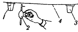
Fig. 157. Checking Radiation Power of Radio Range Finder 1 - transmitting antenna CD-1; 2 - power-level indicator; 3 - receiving antenna; 4 - aircraft skin.
