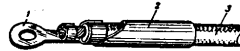
Fig. 31. Terminating of Wire into Lug for Connection to Wet Terminals 1-lug; 2-vinyl chloride tube; 3-wire.
