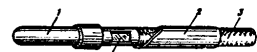
Fig. 33. Terminating of Wire into Connector Plate 1-plate; 2-vinyl chloride tube; 3-wire; 4-strand.
