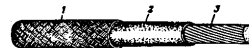
Fig. 28. Wire 5100 1-braiding of cotton yarn coated with micrograph; 2-wire; 3-strand of tinned copper wires.
