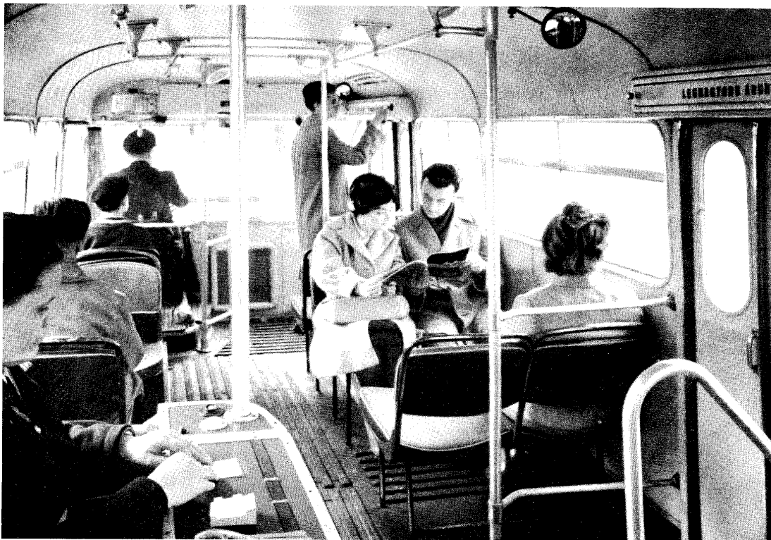
Soft, plastic-lined seats, easy-to-reach grips await passengers in the 11.5 m, excellently sprung bus.
