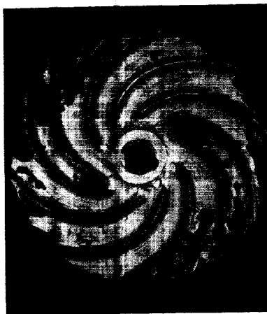
Fig. 17—Pump rotor corroded beyond further use.
