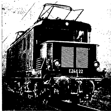
Abb. 2: Lokomotive Bauart Bo'Bo' E 244.22
