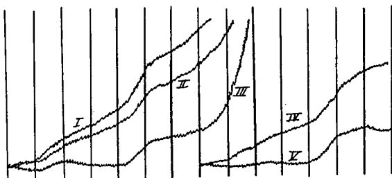
Figure 6. Polarogram of Pb, Taken Without Compensation for Current (curves I, II, IV), and With Compensation for Current (curves III, V)
