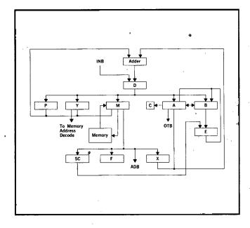
A Register (A) — The A register is a 16-bit register used as the primary arithmetic and logic register of the computer. The A register can be displayed and manually controlled on the computer control panel.
