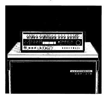
The DDP-516 console is cable-connected to the central computer and can be positioned anywhere on the top of the cabinet to suit operator convenience. Or it can be moved to an adjacent table if preferred.
