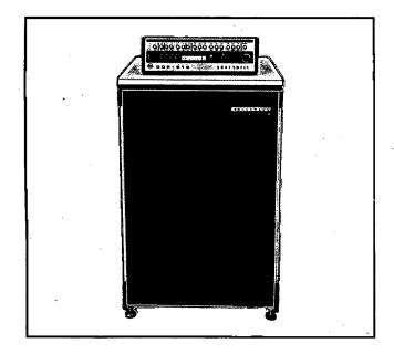
$\mu\text{-COMP}$  DDP-516 is a compact, low cost, high performance 16-bit binary general purpose digital computer. Standard memory capacity is 4096 words (expandable to 32,768) with 0.96  $\mu\text{sec}$  cycle time. Extremely high computation and I/O speeds make the DDP-516 ideal in real-time on-line systems applications.
