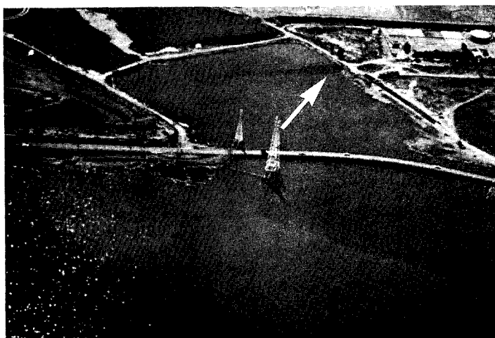
Figure 8.- Sewage treatment plant which discharges into the San Francisco Bay. Mildly stated, this plant has a serious odor problem during warm weather. The tone and color of the receiving waters is an oily gray, an appearance which is characteristic of some badly polluted waters, particularly turbid waters which are low in dissolved oxygen.
