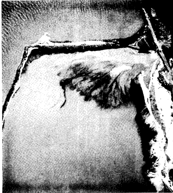
Figure 15.- Arrow points to drainage from hydraulic dredge filling in tidal marsh near Foster City, California. Note sediment pollution.
