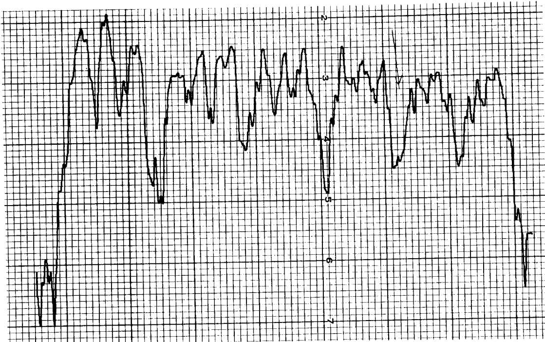
Figure G8. Three-Bar Target Focused with 546 Millimicron Filter and Traced with 546 Millimicron Filter
