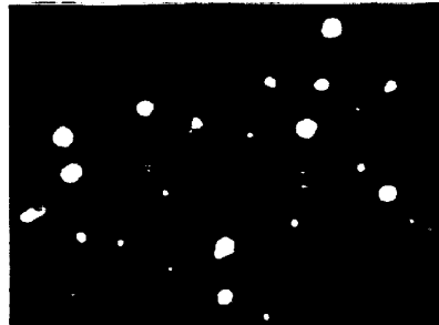
Fig.15: Counting plate for white crepe with 0.004% Inca carbon black. Counted particles 124.
