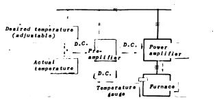
Fig.17: Circuit diagram of a magnetic amplifier for regulating an electrical industrial resistance furnace.
