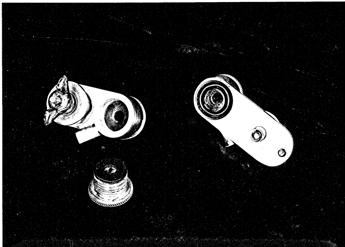
Figure 14. Dust and Water Collector Incorporating a Grease Chamber
