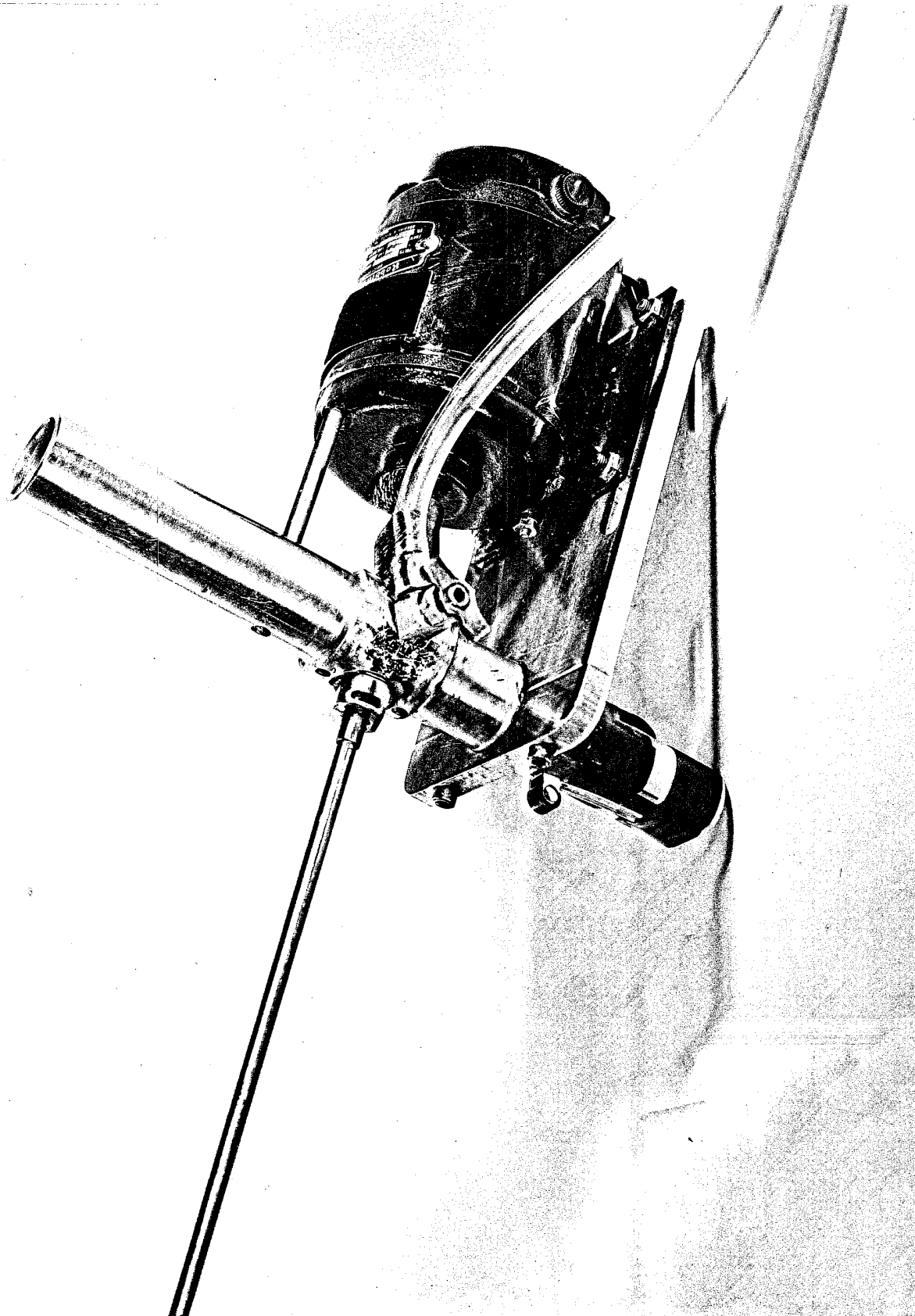
Figure 7. Experimental Hand-Held Drilling Unit
