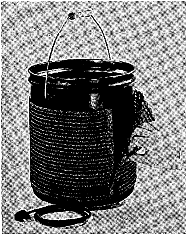
Net contact heater made by Pre-Fab Co. for melting 5-gal drums of plastisol has nylon-reinforced glass cord insulation impregnated with silicone resin varnish. Device was originally developed to keep high altitude aerial cameras and control mechanisms operative in sub-zero environments. (Dow Corning Corp.)
