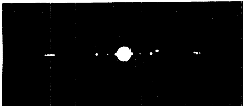
(a) 5X enlargement of the coherent power spectrum of a zone plate containing three discrete electrical noise frequencies.
